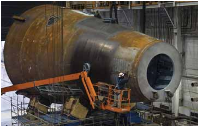
A shipbuilder on a lift works on the stern unit of the USS Indiana at Newport News Shipbuilding in 2013. Photo by Ricky Thompson.
